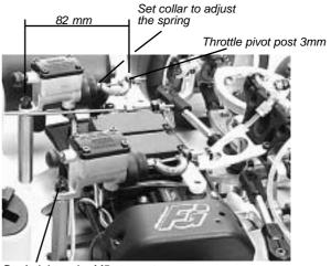
Don't tighten the M5 stop nut. The main brake cylinder should be moveable in every direction.
