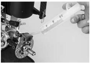
Press the injection with filling hose on the valve. Open the valve and press the hydraulic oil slowly through the brake system.
