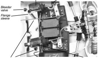
The chassis borings must be placed in linear link to the servo. Bore the chassis with 5,5mm and countersink it with 90° from underneath.
