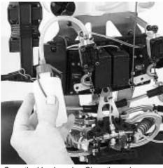
Open the bleeder valve. Close the main brake cylinder completely Collect the overflowing oil at the main brake cylinder with plastic bottle 9452/1.
